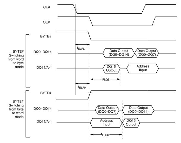
Figure 15. BYTE# Timings for Read Operations
