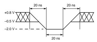
Figure 7. Maximum Negative Overshoot Waveform
