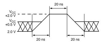
Figure 8. Maximum Positive Overshoot Waveform
