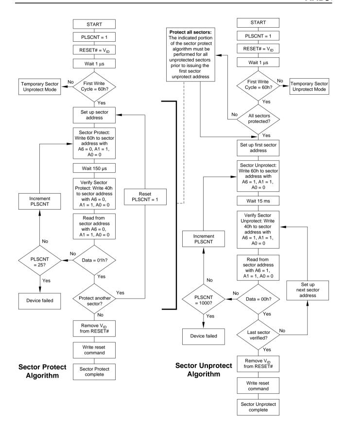
Figure 1. In-System Sector Protect/Unprotect Algorithms
