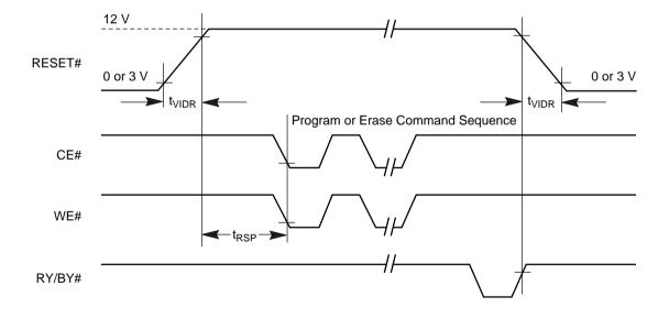
Figure 22. Temporary Sector Unprotect Timing Diagram
